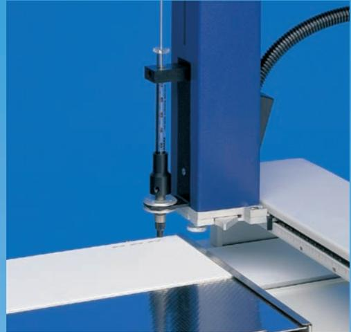
The sample liquid is sprayed onto the layer from the tip of the syringe needle. The stage movement is controlled so that the sample is uniformly distributed over the entire length of the band.
