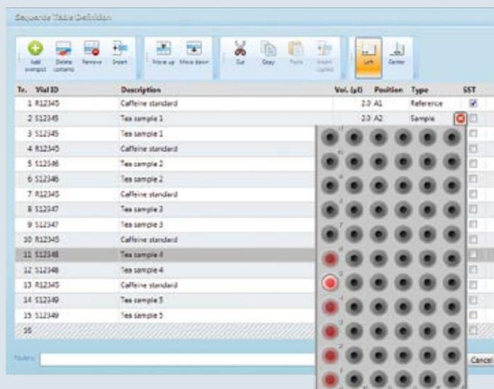
Easy sequence setup with *visionCATS*: the sequence table holds all information required to fully automated run a series of samples, e.g. sample location (rack position and application position), sample volume, sample name, etc.
