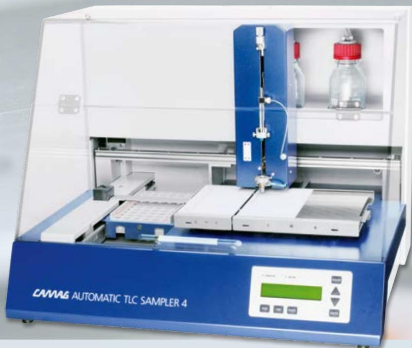
Automatic sample application is a key factor for productivity of the HPTLC laboratory. The ATS 4 offers fully automatic sample application for qualitative and quantitative analyses as well as for preparative separations. It is suited for routine use and high sample throughput.
