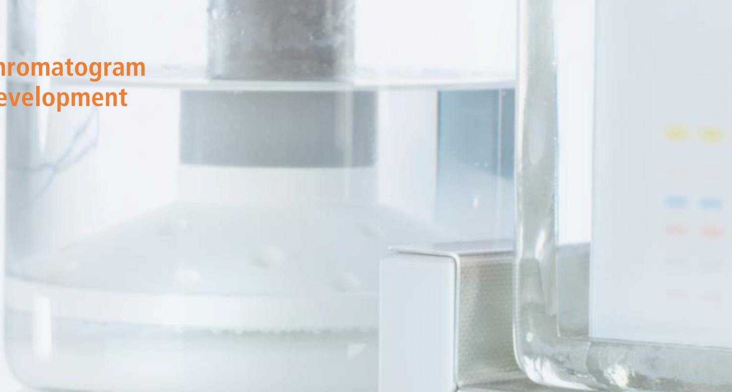
TLC and HPTLC differ from all other chromatographic techniques in the fact that in addition to stationary and mobile phases, a gas phase is present. This gas phase can significantly influence the result of the separation.
