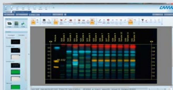
"Data View" allows for visual evaluation of a plate in different illumination modes and offers a broad range of helpful tools, e.g. a  $R_f$  tool displays the  $R_f$  value of zones on the digital image or a rectangular zoom function.
