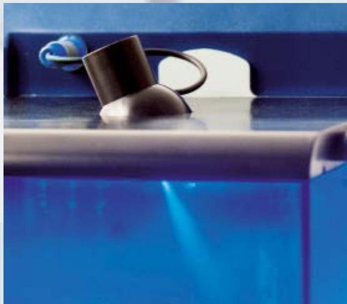
The nozzle generates an extremely fine reagent mist, which evenly distributes in the chamber and gradually condenses on the TLC/HPTLC plate.
