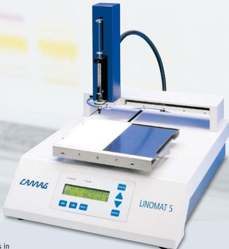
With the Linomat 5 samples are sprayed onto TLC/HPTLC plates in the form of bands with nitrogen or compressed air. Sample application is automatic, only changing the syringe (filling, inserting and rinsing) is manual. The Linomat is suitable for small sample throughput.
