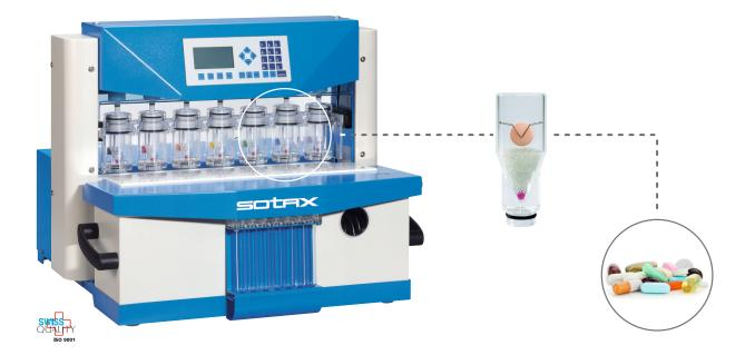
SOTAX CE7 Smart (USP4 Flow Through Cell) Allows you to see differences in your formulations that apparatus 1 and 2 simply do not show. Also widely recommended for poorly soluble, modified / extended release, and low dose products; Also been used for IVIVC studies and a growing range of dosage types
